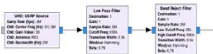
Figure 3: Band filtering to obtain narrow RX window
