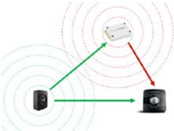
Figure 2: MyQ state sensor broadcasts valid signals (green) while the USRP broadcasts an on-demand jamming signal (red)
