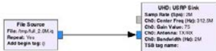
Figure 6: Signal replay flow
